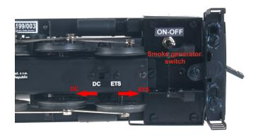
The underside of the locomotive has a switch for selecting operating modes. In the left position, marked "DC", the locomotive runs on DC voltage 0-18V. In the right position, marked "ETS", the locomotive runs using the ETS impulse controller (ETS model 702 or 702N), which supports the sound generator and allows remote control of the whistle.
